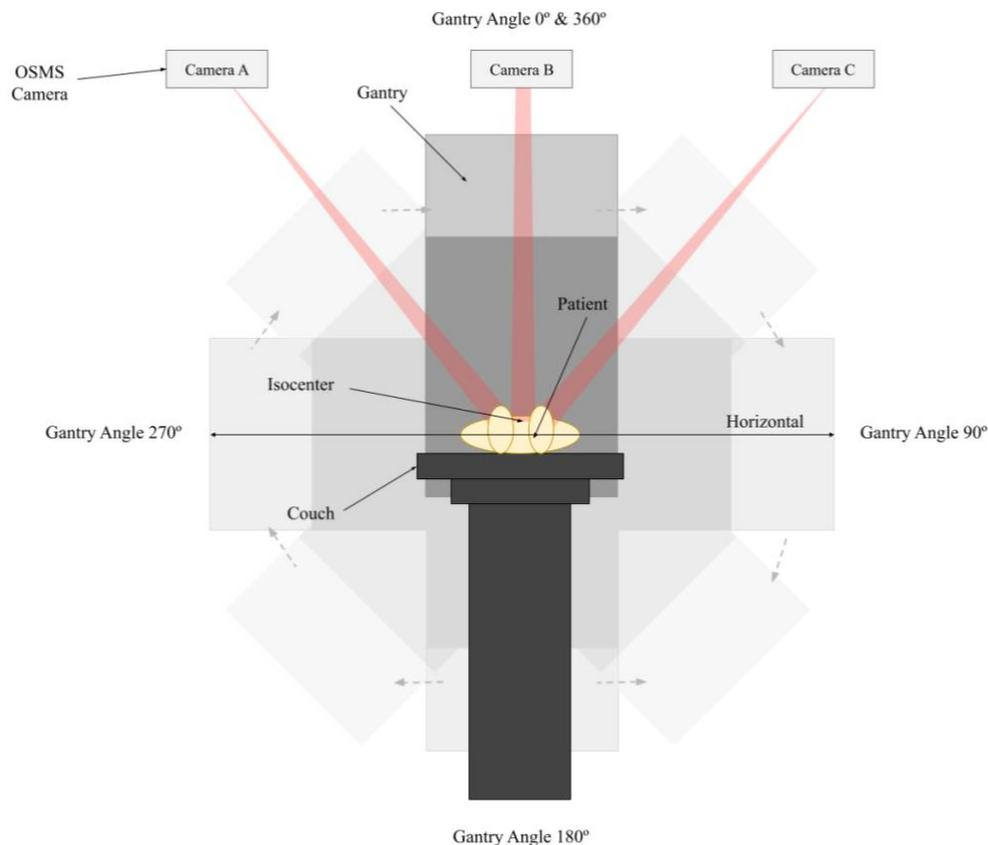
**Figure 3.** Schematic Diagram of Gantry Angles and OSMS Camera Positioning during VMAT. The optical surface monitoring system incorporates three cameras designated as Cameras A, B, and C. Each camera is mounted to the ceiling. Camera B is offset from the plane of the image towards the viewer. The gantry cannot rotate beyond 180° from the 0° or 360° position. Thus, its movement is as follows: 0° → 90° → 180° → 90° → 0° → 270° → 180° → 270° → 360°. This figure was created using Google Drawings.
